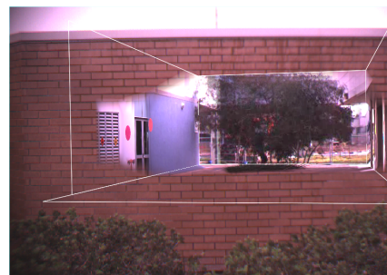
Figure 2 – Our old AR x-ray vision system did little to convey depth. The x-ray images appeared to be floating in front of the walls, rather than behind.
