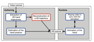
Figure 2: The pipeline of TutAR. Automated steps are colored blue, whereas steps which require author input are colored red.
