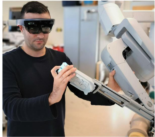
Fig. 1. AR-assisted robot arm positioning.
