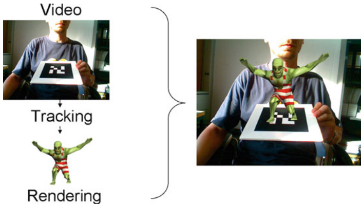
Fig. 3.1 Data flow in a common AR system. Real world imagery is delivered by the system's video feed and processed by vision based tracking algorithms. To align virtual and real data, the derived tracking data has been applied to transform the virtual content. Finally, the rendering is overlaid on top of the video feed
