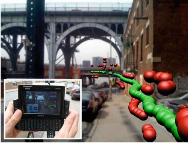
Fig. 3.21 Sitelens. Colored spheres represent geocoded sensor data that is invisible to the eye
