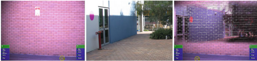
Fig. 3.11 The Augmented Reality system uses a priorly acquired textured reconstruction of a remote scene ( center ) based on captured images and derived models. The textured reconstruction is overlaid on the user's view of the environment ( left ). In combination with highlighting the edges of occluding structure, only where hidden elements can be revealed, a comprehensible x-ray visualization is achieved while at the same time edge clutter is avoided ( right )
