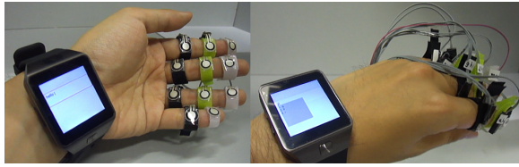
Figure 3: Experimental prototype, typing in hand up (left) and hand down (right) condition
