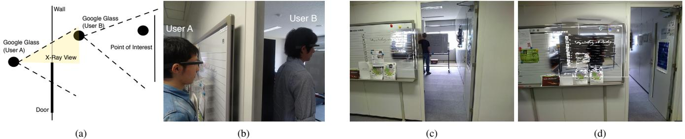
**Figure 1:** In our demonstration users A and B are separated by a wall, both wearing a Google Glass. User A views a point of interest, currently only visible to user B ((a) and (b)). User A's view is augmented with video streamed from user B when the target is partially (c) or fully (d) occluded. (Note: (c) and (d) contain simulated augmentations)
