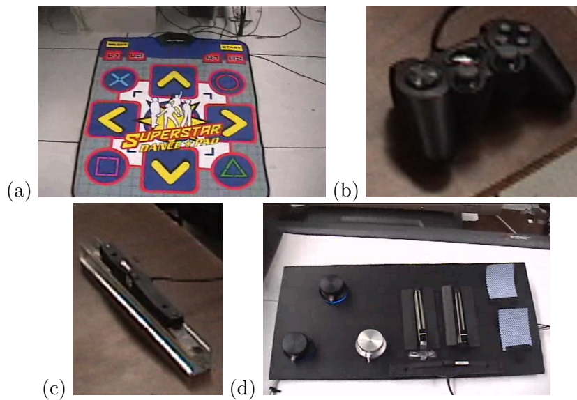
Figure 5.13: Input devices used in our prototype: (a) Dance mat. (b) Game controller. (c) Wand with attached InterSense 6DOF tracker. (d) Tracked board with PowerMate sensors (left) and MIDI sensors (right): sliders and bend sensors attached to playing cards.
