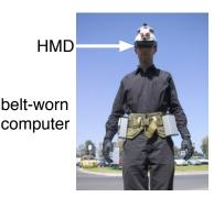
Figure 3. TINMITH: Our previous high-fidelity prototyping platform for AR with a headmounted display (HMD).
