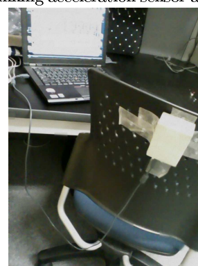
Fig.1 linking acceleration sensor and Arduino
